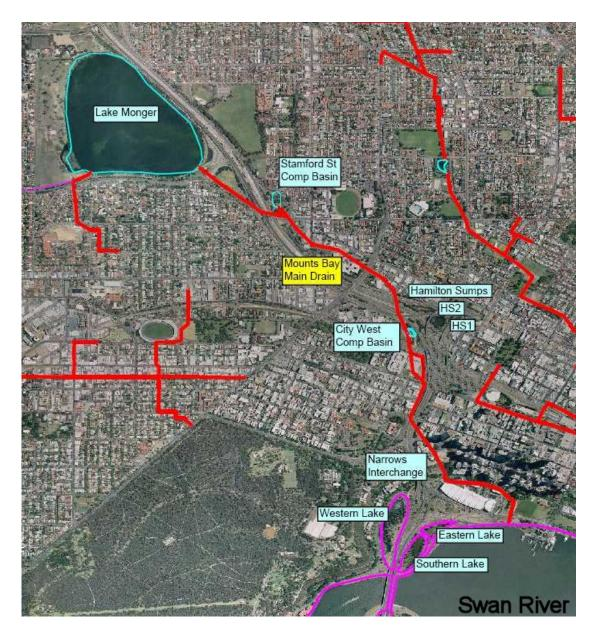
The Mounts Bay Drain was constructed in 1909 to connect Lake Monger to the Swan River, allowing water levels in Lake Monger to be regulated. Overflow from Lake Monger, flows via the Mounts Bay Main Drain, discharging into the Swan River at Mounts Bay through an outlet west of Barrack Square. Between Lake Monger and the Swan River, water bodies at Stamford St and Citywest (west of the Hamilton Interchange) act as compensating sumps. These are controlled by the Water Corporation.
